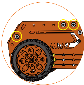
Left side panel installation diagram (Right side panel is the same)
